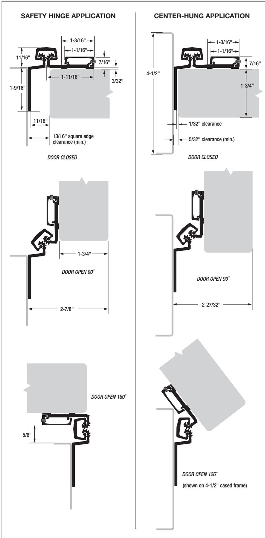
**MATERIAL:** Extruded 6063 T6 aluminum alloy with self-lubricating polyester thrust bearings.
