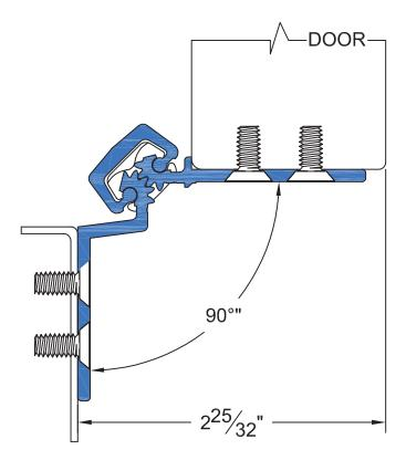
A FRAME WITHOUT A STOP ON THE HINGE MOUNTING SIDE OF THE JAMB MUST BE USED IN CONJUNCTION WITH THE SL71 FOR THE SAFETY FEATURE TO BE EFFECTIVE.
