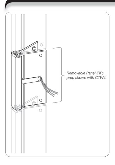
**PREP:** SELECT geared continuous hinges can be prepared with removable hinge leaf panels to allow easy access and service of electrical components without removing the door.
