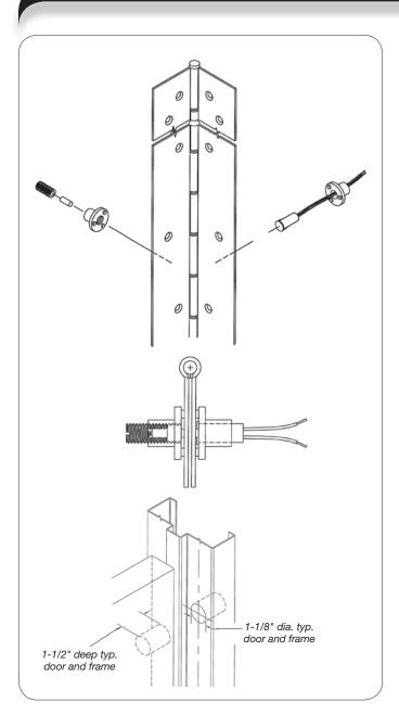
PREP: SELECT pin & barrel continuous hinges can be prepared for the adjustable concealed monitor switch. Rigid welded assembly gives you the ability to adjust the AMS to work with all applications.
